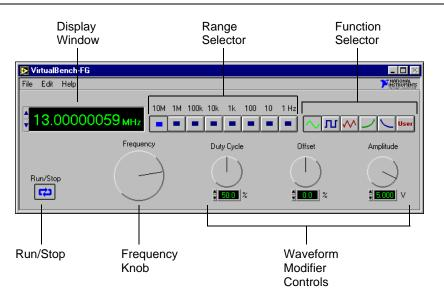
The front panel of VirtualBench-FG has the following features:
